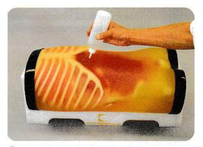
② Spread ultrasound gel over the phantom body.
